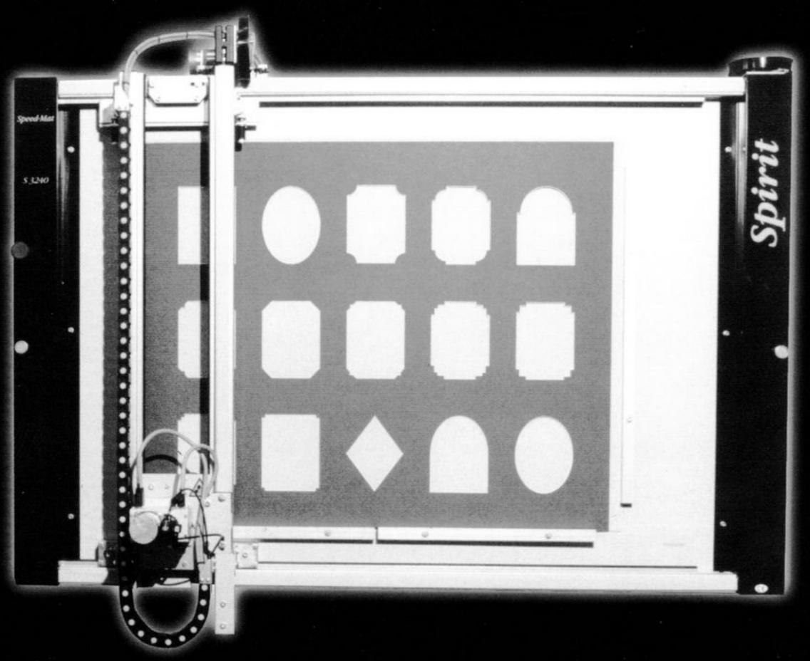
The Speed-Mat Spirit is a state of the art automated mat cutting priced affordably for the custom picture framer. The Spirit will provide a major improvement in efficiency for cutting standard rectangles, ovals, circles and makes it easy to cut more complex shapes.
